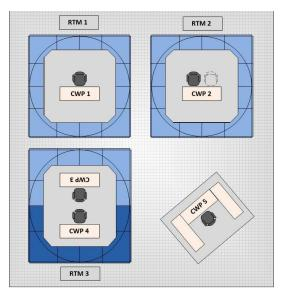
Figure 5 – Potential configurations of the RTM
